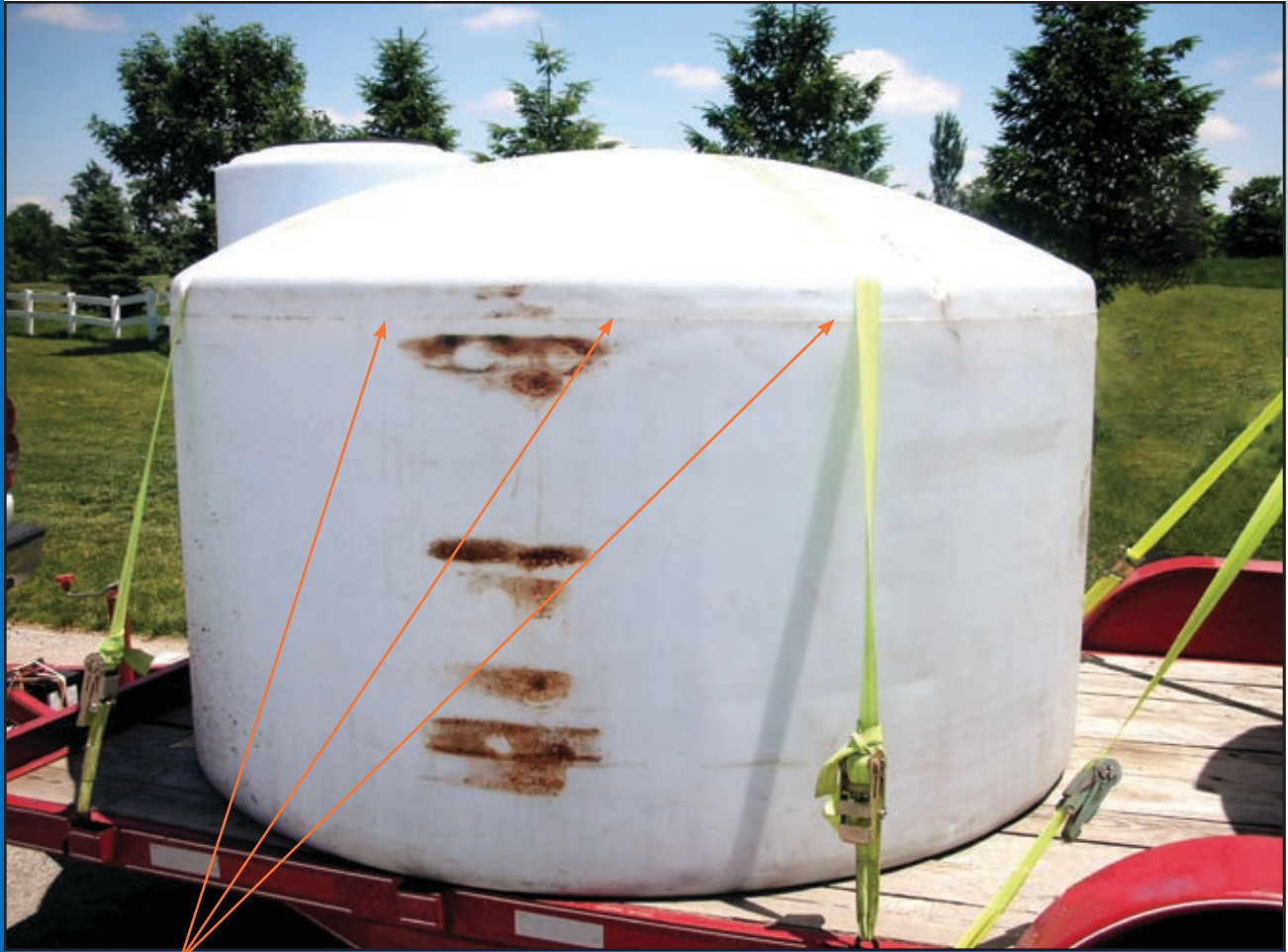
Notice the parting line on this tank.
