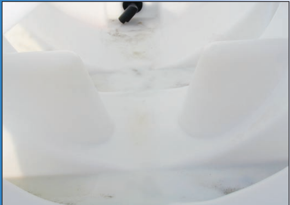
A view inside a transport tank (right), showing the baffles that help control liquid contents during transport.
