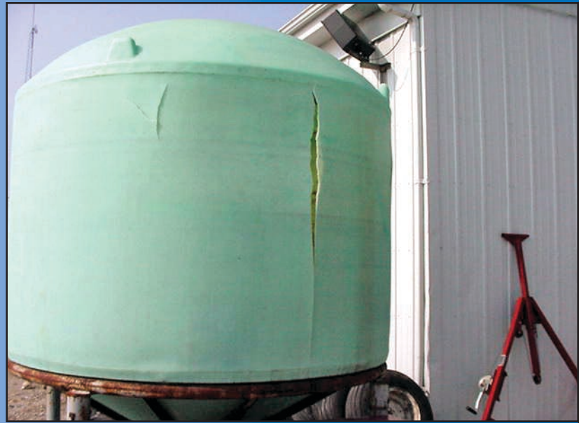
Tanks left outdoors are subject to more sunlight degradation and weathering than tanks kept indoors.
