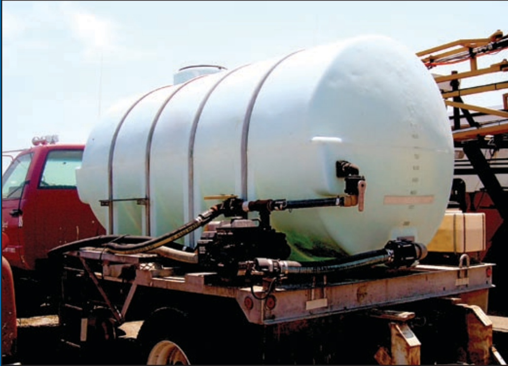
The transport tank (left) has legs and is secured onto the bed of the truck with metal tie-down hoops.
