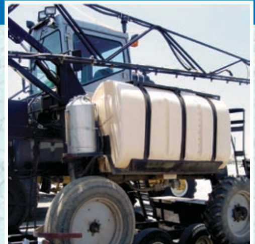
Above: A poly tank used to carry product on a sprayer.
