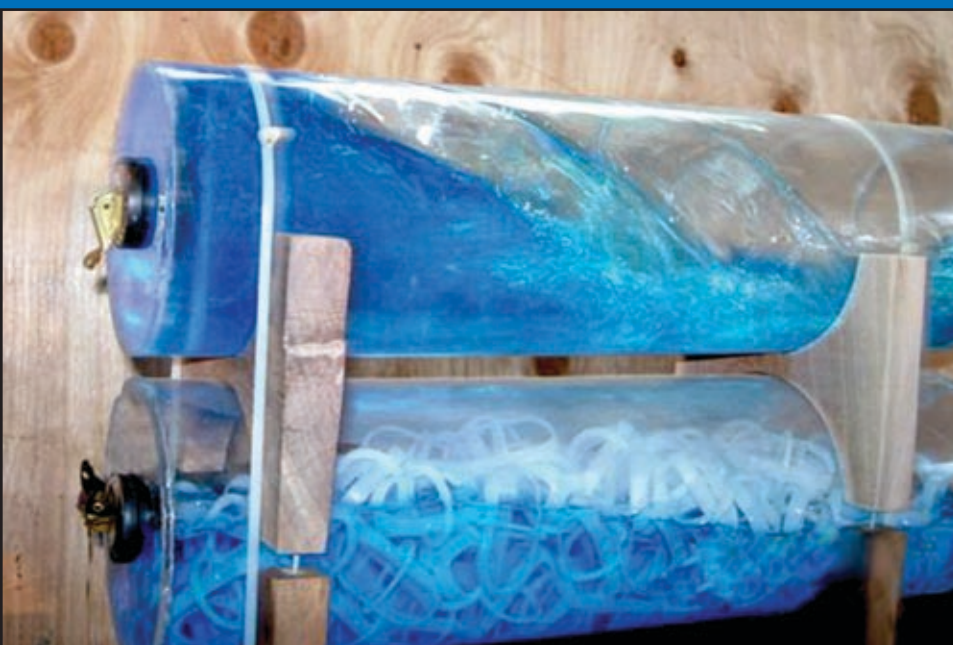
Baffles reduce liquid surge.
