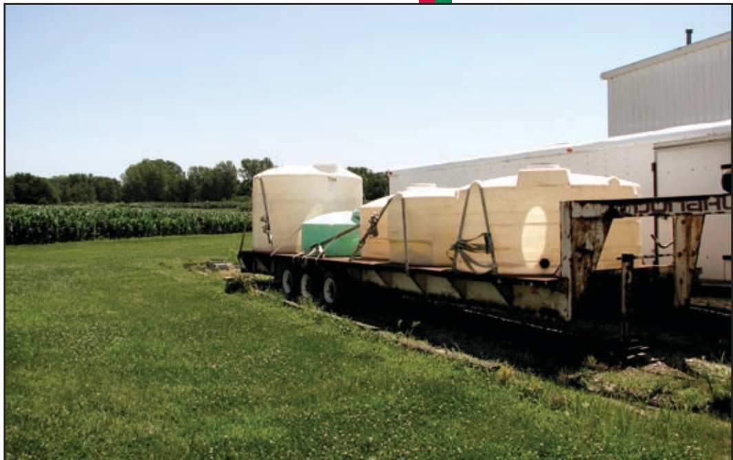
The storage tanks in this photo are being misused as transport tanks.
