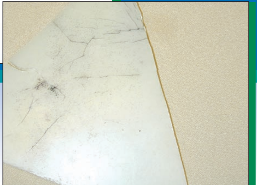
Above: Good, clear plastic without marks. Right: Degraded plastic showing crazing and cracking.
