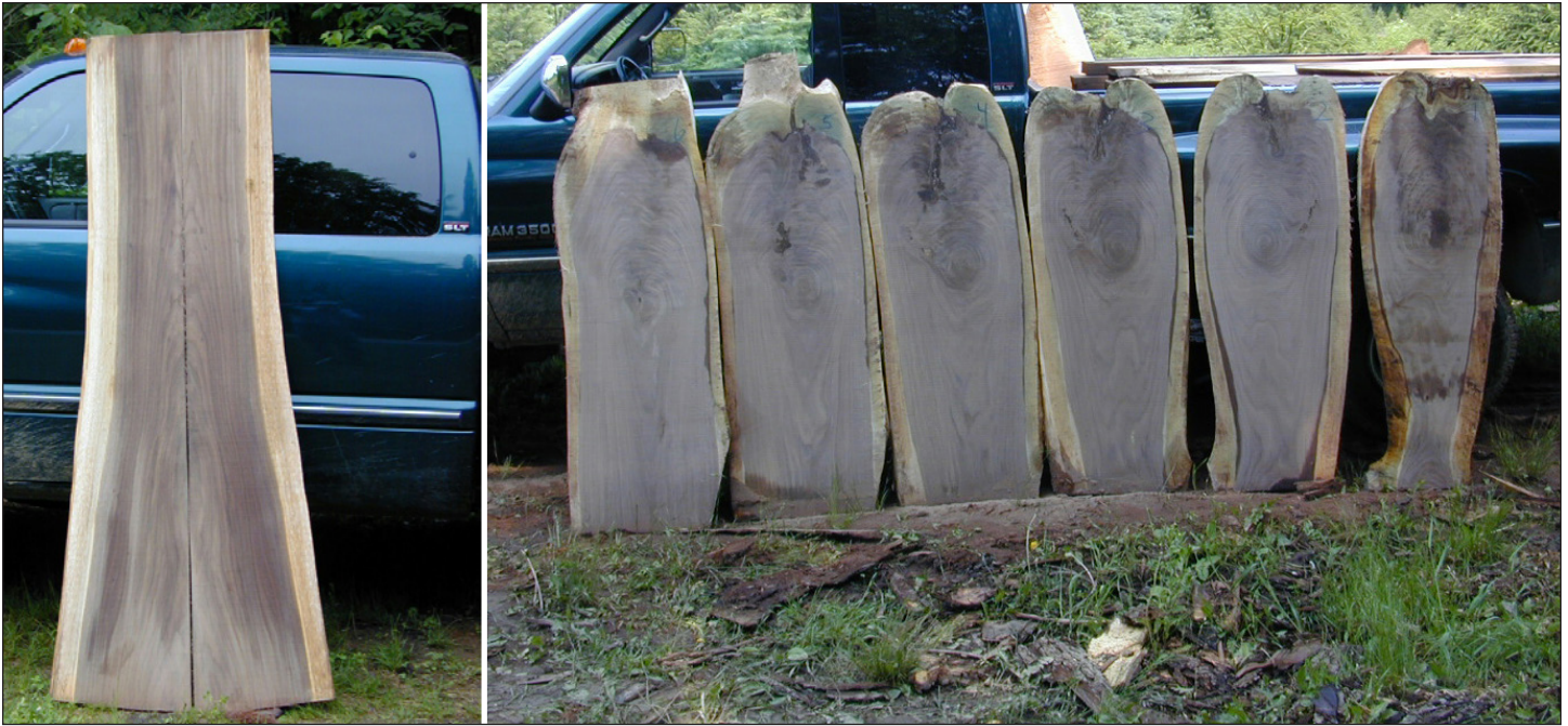
Figure 2. Book-matched walnut slabs (left) and also several pieces of figured walnut from a large crotch produced by a portable thin kerf band mill. Due to production costs, especially labor, most traditional mills will not produce these types of products.
