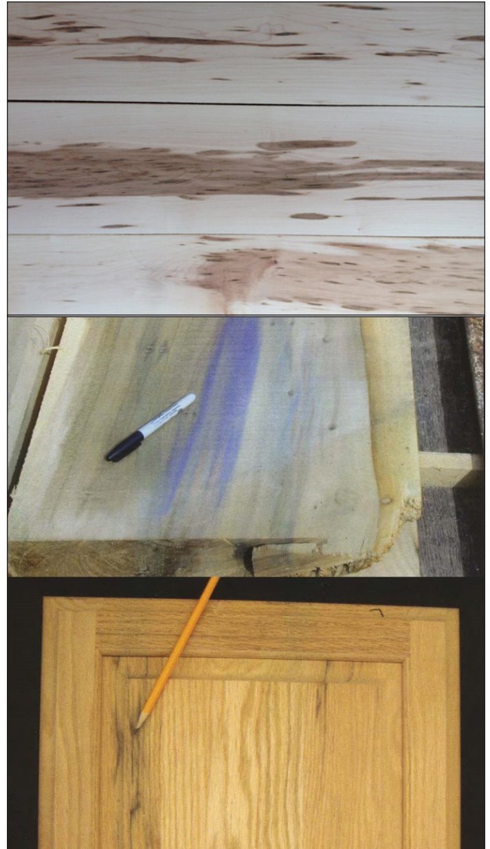
Figure 4. Mineral stain in hard maple (top), yellow poplar (middle) and in red oak (bottom). The white sapwood and brown heartwood of spalted maple is shown in Figure 9.
