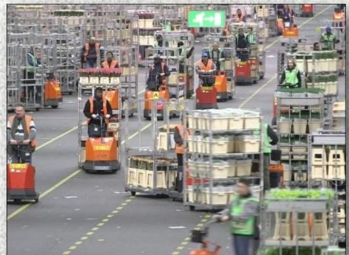
Orange electric tractor units pull trolleys of flowers from the incoming delivery area to the shipping area after purchase.
