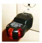
This tool will let you know if voltage is present without physical contact and can detect varying levels of voltage. Test the detector by rubbing it through your hair or on a cloth to create a static electrical charge. You can also insert it into a wall outlet you know is hot. It will light up and beep when it finds voltage. By knowing how it works, you can use it on an unknown circuit to see if the circuit is energized or not.
