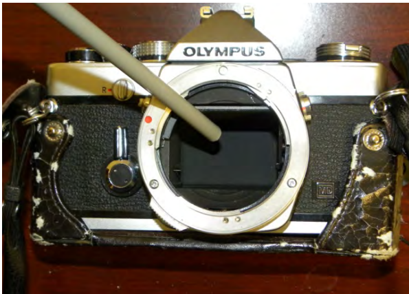
Figure 3. The shutter, which is the sliding screen, on this older film camera is capable of opening and shutting at 1/1000^{\text{th}} of a second
