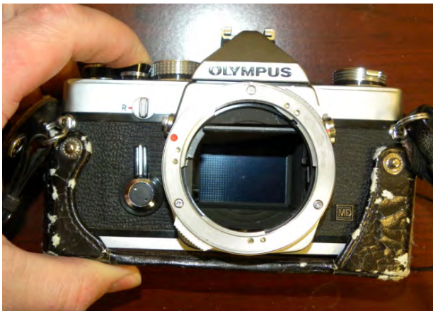
Figure 4. The shiny surface on this old camera was where a roll of film was placed. A sensor is located there on a digital camera that records the image.
