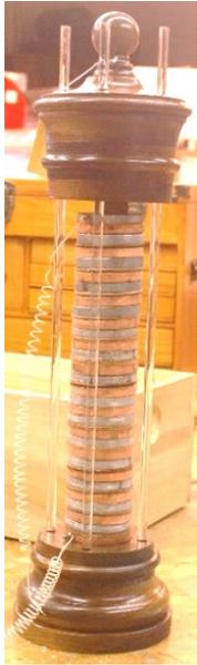
The first practical battery was made by the Italian, Alessandro Volta, in 1799. *Guess where we got the word volt.* He stacked copper washers and cloth washers, soaked in a mild acid, and zinc washers on top of each other to produce a battery of about 30-Volts. Larger diameter washers provide more surface area for more amps of current for more power.
