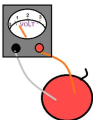
wire or nail, and a shiny copper wire to make this cell. Stick the wires deep in the apple.
