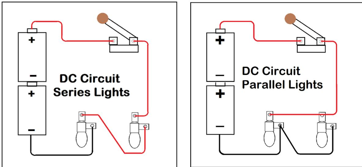
**For the series circuit,** each light bulb (same size) gets 1-1/2-Volts. (The lights will be dim because they are 3-Volt bulbs.) If one bulb is removed the other bulb will go out. The same current (amps) passes through each bulb.
