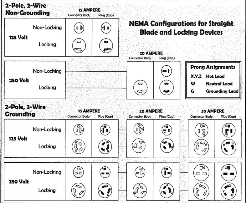
The National Electrical Manufacturers Association (NEMA) has assigned designators to the various configurations. The purpose of so many different types is to prevent the wrong combinations of electrical systems from being plugged together, thereby avoiding potentially dangerous conditions.
