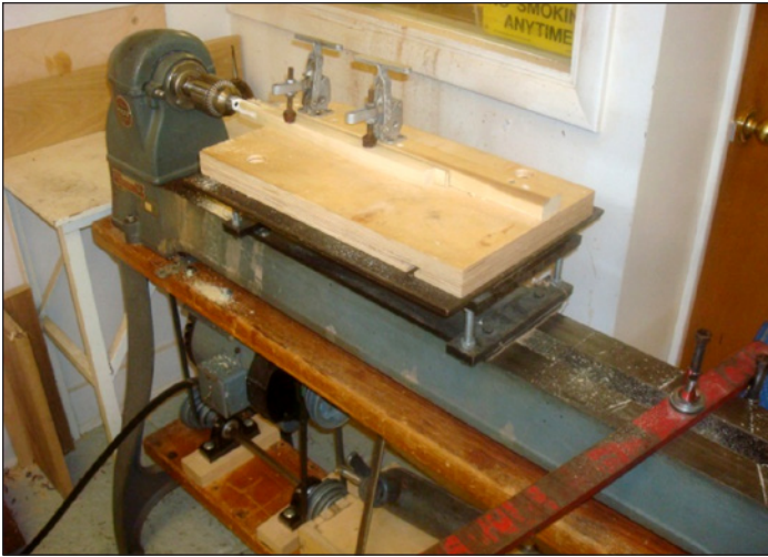
Lathe with table setup to cut tenons
