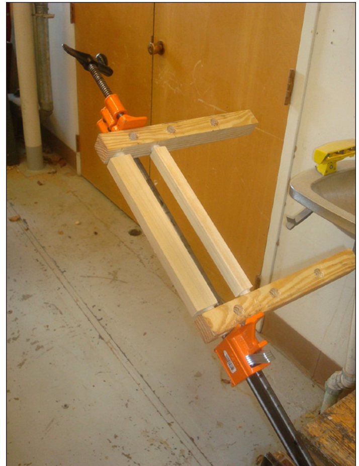
Bar clamp used to incrementally bring legs together
