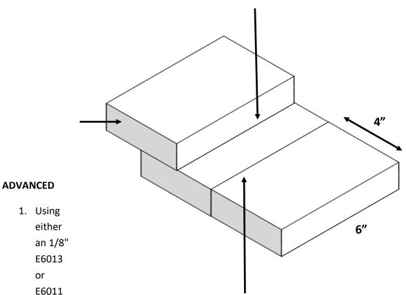
electrode, repeat exhibit specifications from Intermediate Division and add a fourth piece of mild steel with the same dimensions to create a vertical t-weld on top of the lap weld, going up on both sides of t-weld (as opposed to welding down). See "Advanced Diagram" for example.
